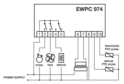
dbi = delay betw. two successive starts. Limits the number of start-ups per hour.
